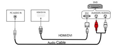
Connect TV with corresponding jacks on DVD or STB, and switch the source to HDMI in Source menu. (Picture A/B)
