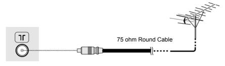
\*If you have a 75 ohm round cable, insert the bronze wire and then tighten the connection nut.
